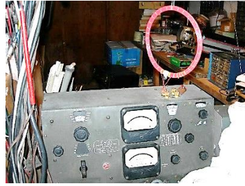
The coil suspended over the Q-meter
