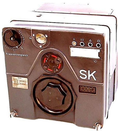
The “Russian” FuGe-10-SK 300-600 kHz, or 3–6 MHz German military transmitter with the original German paint job. FuGe: Funkgerät – radio.
