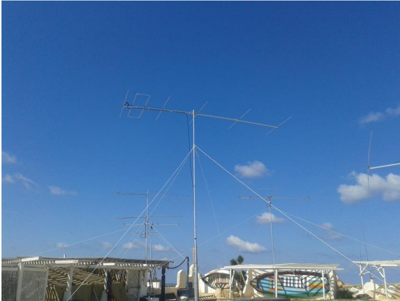
3 70MHz beam a 6 element LFA yagi from EAntenna
